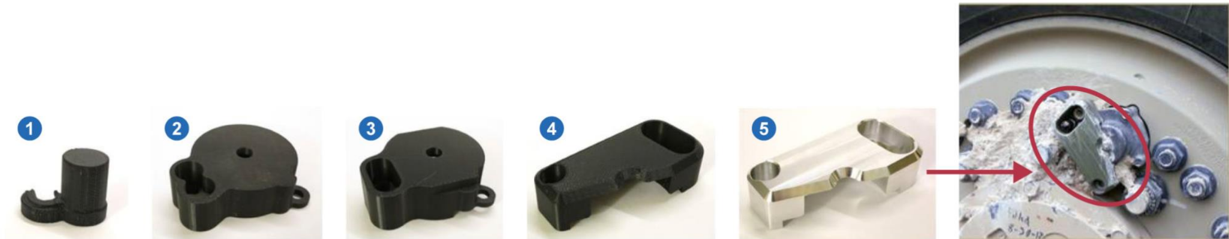
Figure 5: Army Valve Stem Cover Additively Manufactured for Interim Solution
